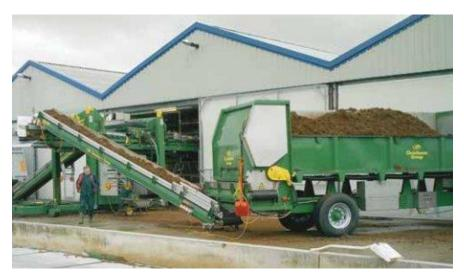
The speed of the dispensing roller at the bottom of the hopper will need to be adjusted so that the 1% dosage can be achieved accurately. NOTE Organic Gold is much finer that other products in the industry so that the mycelium feeds more efficiently. Keep monitoring dispensing as the growing room is being filled to ensure uniform dosing, hopper are notorious for giving variable application rates.
